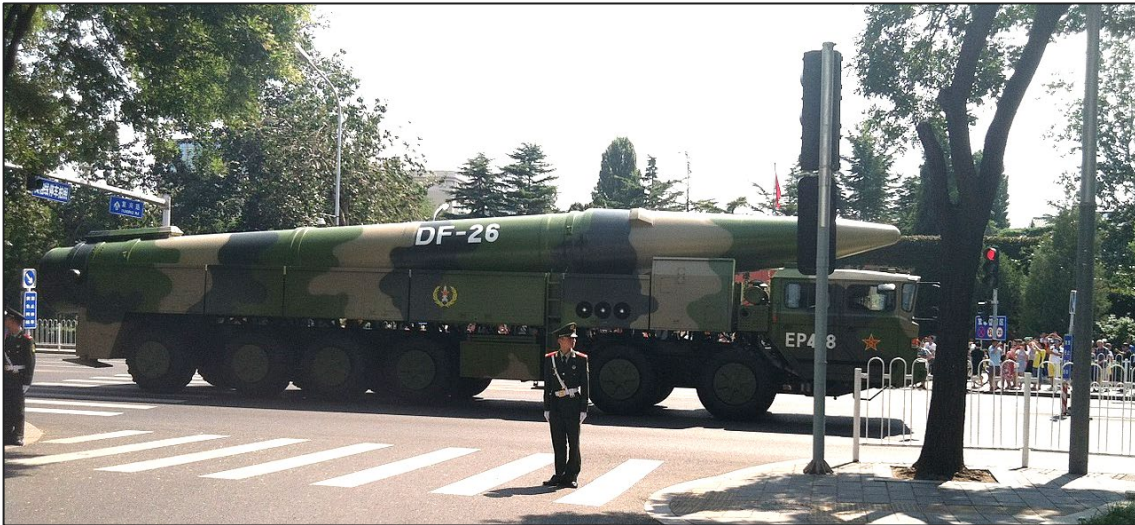
Figure 2.5 The TEL for the DF-26 intermediate-range ballistic missile as seen after the 2015 military parade in Beijing to commemorate the 70th anniversary of the end of WWII. This was the first public display of the DF-26 [20]. China may have up to about 100 operational DF-26 launchers, most of them presumably having a non-nuclear mission [18]. (Photo from Wikimedia Commons, CC BY-SA 4.0 .)
