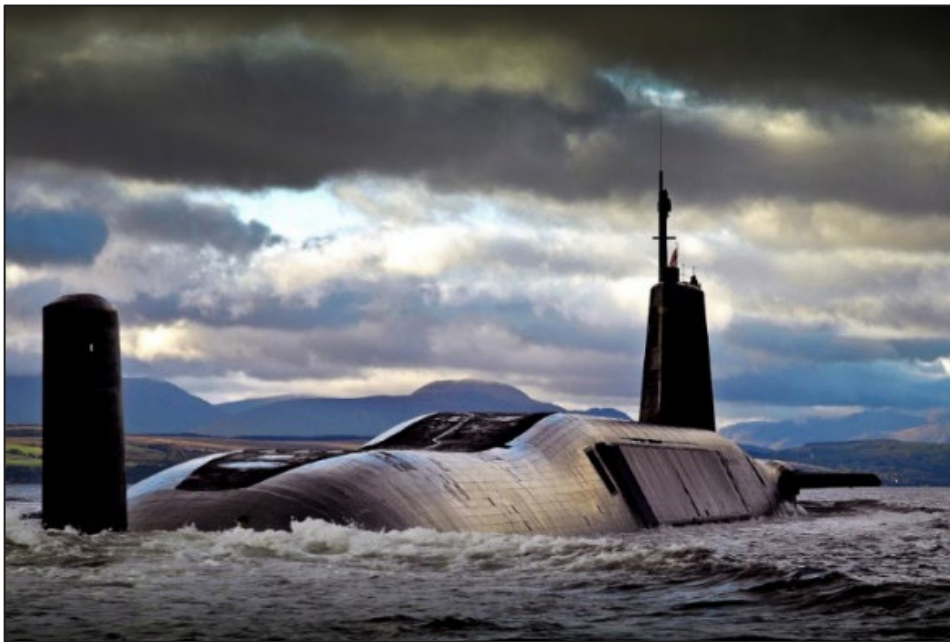
Figure 2.3 The British strategic, nuclear-propelled submarine HMS Vengeance. The United Kingdom has four such submarines, each capable of carrying up to 16 Trident II D5 missiles, each with up to five nuclear warheads. The British government has limited the total number of warheads on a given submarine to 40. [12] (Photo from Wikimedia Commons, courtesy of the Royal Navy, OGL v1.0. )
