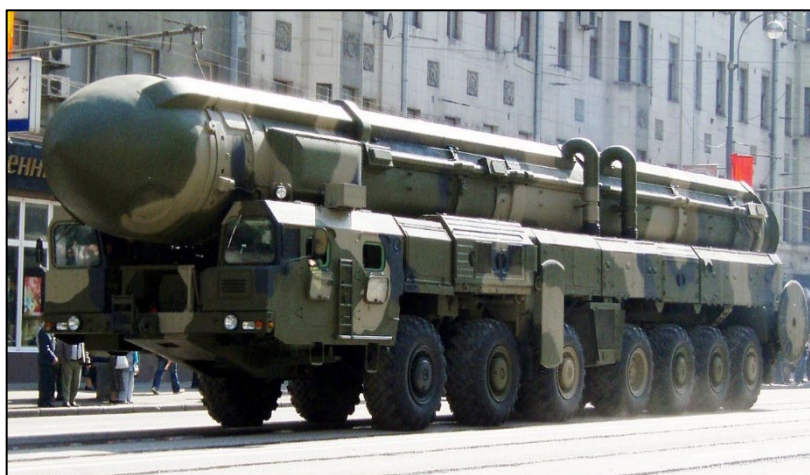
Figure 2.2 A so-called transporter-erector-launcher (TEL) for a Russian intercontinental ballistic missile photographed in a Moscow street in 2008. The launcher may or may not contain its designated missile, referred to as Topol in Russia and SS-25 Sickle in NATO. It carries only one nuclear warhead, weighs about 45 metric tons at launch, is 20.5 m long and has a range of 11 000 km [10]. (Photo from Wikimedia Commons, CC BY-SA 3.0 .)
