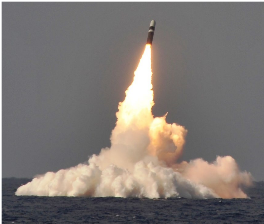
Figure 2.1 Test launch of a Trident II intercontinental ballistic missile from the Ohio class strategic submarine USS West Virginia. All U.S. SLBMs are of this type. (Photo from Wikimedia Commons, U.S. Navy work, Public Domain.)
