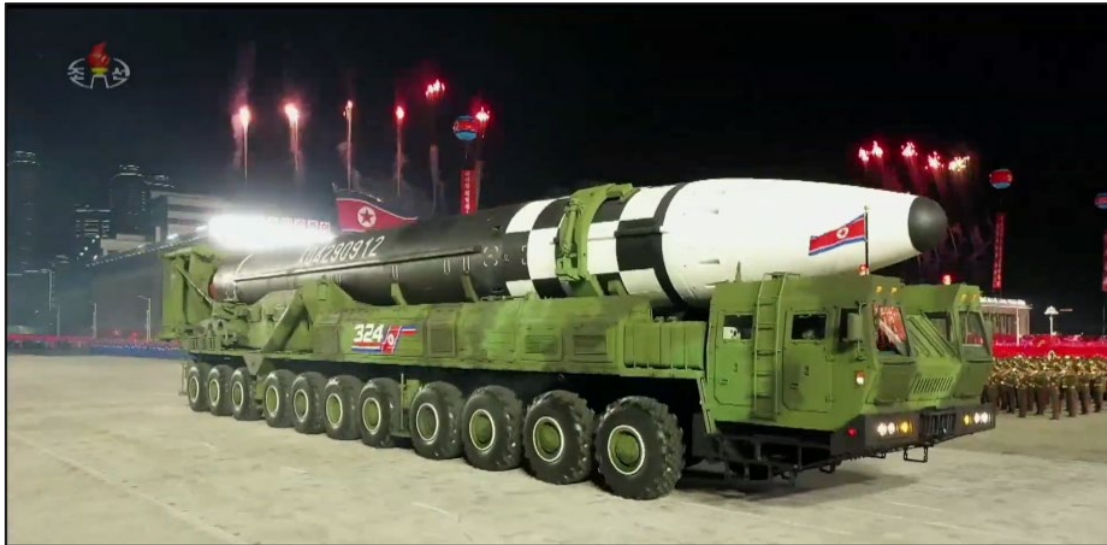
Figure 2.8 A road-mobile ICBM, tentatively called Hwasong-16, debuting in the public during a parade in Pyongyang in October 2020. (Photo from Wikimedia Commons, screenshot from KCTV.)
