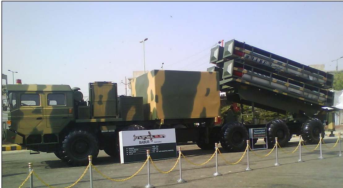
Figure 2.7 The launcher for the Pakistani Babur (Hatf-7) ground-launched nuclear cruise missile photographed in 2008. The launcher carries four missiles with wings unfolding after launch as shown on the sketch in front of the vehicle. (Photo from Wikimedia Commons, CC BY-SA 3.0 .)
