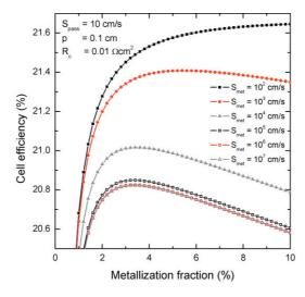
Fig. 5. Simulated cell efficiency of a PERC-type Si solar cell as a function of the rear side metallization fraction for different values of the SRV of the metallized area  $S_{met}$ . Values for the SRV of the passivated area  $S_{pass}$ , the contact pitch p and the area-specific contact resistance  $R_c$  are indicated. (Setup time:  $\sim$ 30 s. Simulation time:  $\sim$ 1 min).
