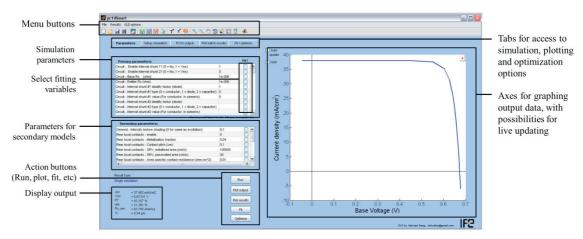
Fig. 2. Illustration of the graphical user interface at the time of writing. Several relevant features of the program are indicated.
