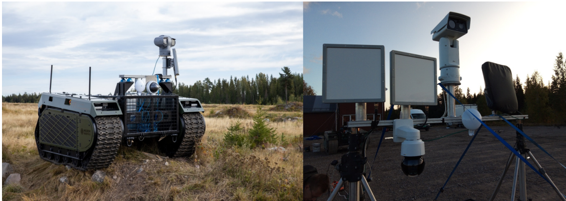
Figure 2.5 The two Sentry platforms at LandX20. To the left, the remote sentry is shown mounted on a UGV, to serve as an autonomous forward observer. To the right, the main Sentry platform is shown.
