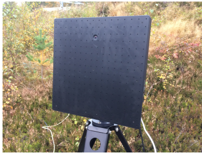
Figure 2.9 Discovair G1 sensor panel (left) and the web-cam image showing the grid layout and examples of tracked drones (right).
