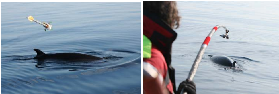
Tag deployment systems: The ARTS system (left) and the hand held pole (right) used to deploy DTAGs. When deploying the tag with the ARTS the tagger shoots from the elevated platform in the bow of tag boat 2. The pole techniques will primarily be used from tag boat 1.
