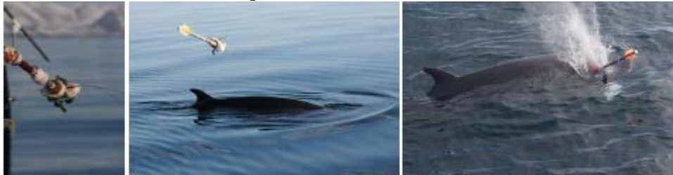
The ARTS system (left) used to deploy a DTAG (middle) and a CTAG (right) on minke whales.
