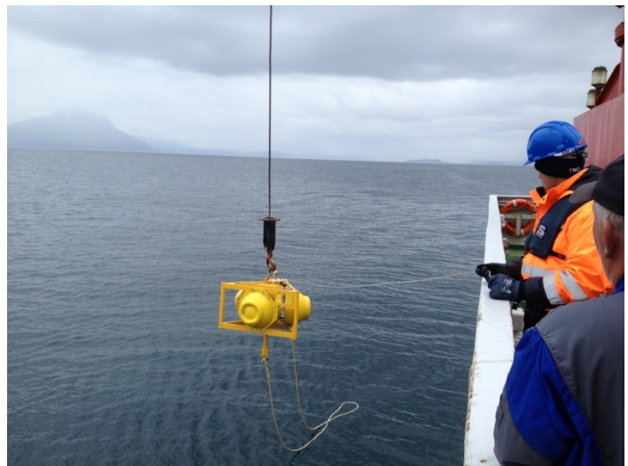
Figure 3.19 Configuration of the sonar buoy used during 3S-2013 (left). Positions of the hydrophones are marked A, C and D. Deployment of the buoy (above), the hydrophones are attached at a later stage using one of the tag boats (photo F.P. Lam).
