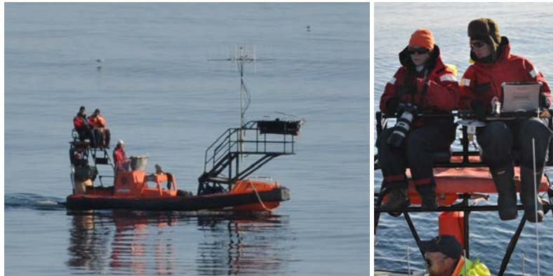
The MOBHUS/tag boat 2 tracking boat equipped with an elevated observation platform (right) and antennas for radio tracking of the tag.
