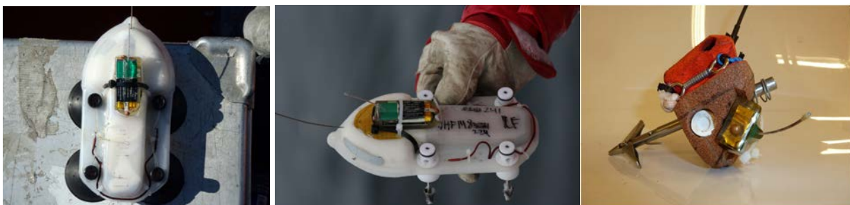
DTAG2 with suction cups (left), DTAG2 with small 50mm invasive barbs (middle), and CTAG (right). All tags will have a Sirtrack GPS logger piggybacked to them.
