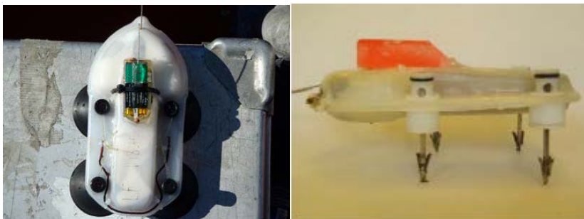
DTAG2 with suction cups (left) and with small 55 mm invasive barbs (right). Both tags will also have a GPS logger piggybacked to them.
