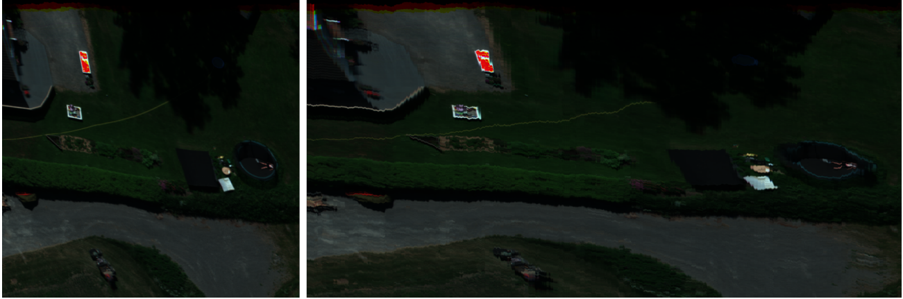
Figure 8. Reconstructed (R, G, B) push broom image based on VSLAM + global mesh with (left) and without (right) our stabilisation approach.
