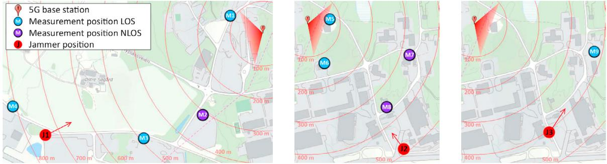
Fig. 2. (a) measurement positions M1–M4 and jammer position J1, uplink jamming; (b) measurement positions M5–M8 and jammer position J2, uplink jamming; (c) measurement position M9 and jammer position J3, downlink jamming.
