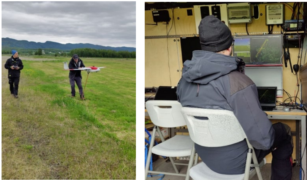
Figure 2.2 The aircraft was launched from a customized launching devise (left), and monitored from a mobile ground control station (right).
