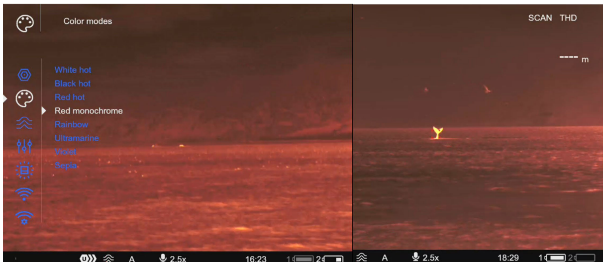
Figure 6. Test of Pulsar Merger LRF XP50 in total darkness. In the left panel humpback whales at 1,600 m by using red monochrome colour mode, while in the right panel a humpback whale tail at 1,000 m by using red monochrome colour mode.
