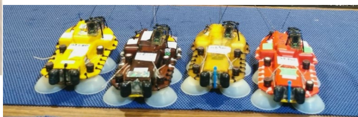
Figure 2.2 Left: Mixed-DTAG ++ used in the 3S-2023 research trial. Note the suction cups used to attach the device to the skin of the whales. The DTAG3 core unit logs audio and movement of the tagged whale and operates the tag-release system via tygon tubes attached to each suction cup. The Little Leonardo video-data sensor records wide-angle video as well as 24-hours of depth and 3-axis accelerometer data. The LOTEK GPS-ARGOS unit records GPS signals, which are logged and then transmitted to the ARGOS satellite system. A LOTEK V7G 149A VHF transmitter is used to assist tagged whale tracking and for tag recovery. Sufficient flotation is included to enable good positive buoyancy of the device. Below: Four mixed-DTAG ++ units ready for deployment during the 3S-2023 research trial.
