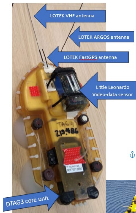
Figure 2.2 Left: Mixed-DTAG ++ used in the 3S-2023 research trial. Note the suction cups used to attach the device to the skin of the whales. The DTAG3 core unit logs audio and movement of the tagged whale and operates the tag-release system via tygon tubes attached to each suction cup. The Little Leonardo video-data sensor records wide-angle video as well as 24-hours of depth and 3-axis accelerometer data. The LOTEK GPS-ARGOS unit records GPS signals, which are logged and then transmitted to the ARGOS satellite system. A LOTEK V7G 149A VHF transmitter is used to assist tagged whale tracking and for tag recovery. Sufficient flotation is included to enable good positive buoyancy of the device. Below: Four mixed-DTAG ++ units ready for deployment during the 3S-2023 research trial.
