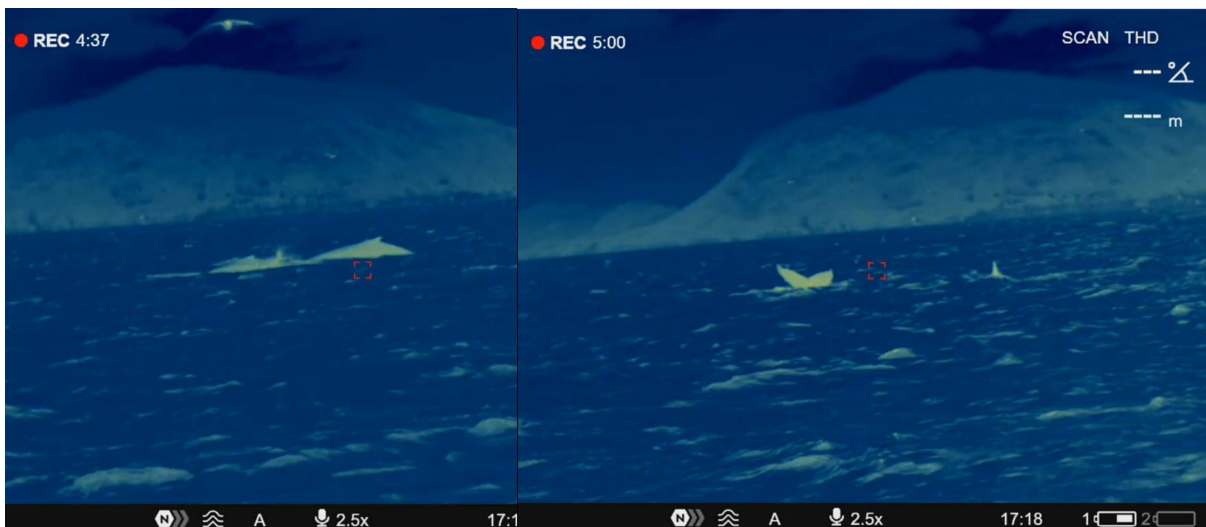
Figure 1. Test of Pulsar Merger LRF XP50 in total darkness. In the left panel humpback whales are visible at 300m, while in the right panel humpback whale tail and a killer whale are visible at 300m, both by using Ultra marine colour mode.
