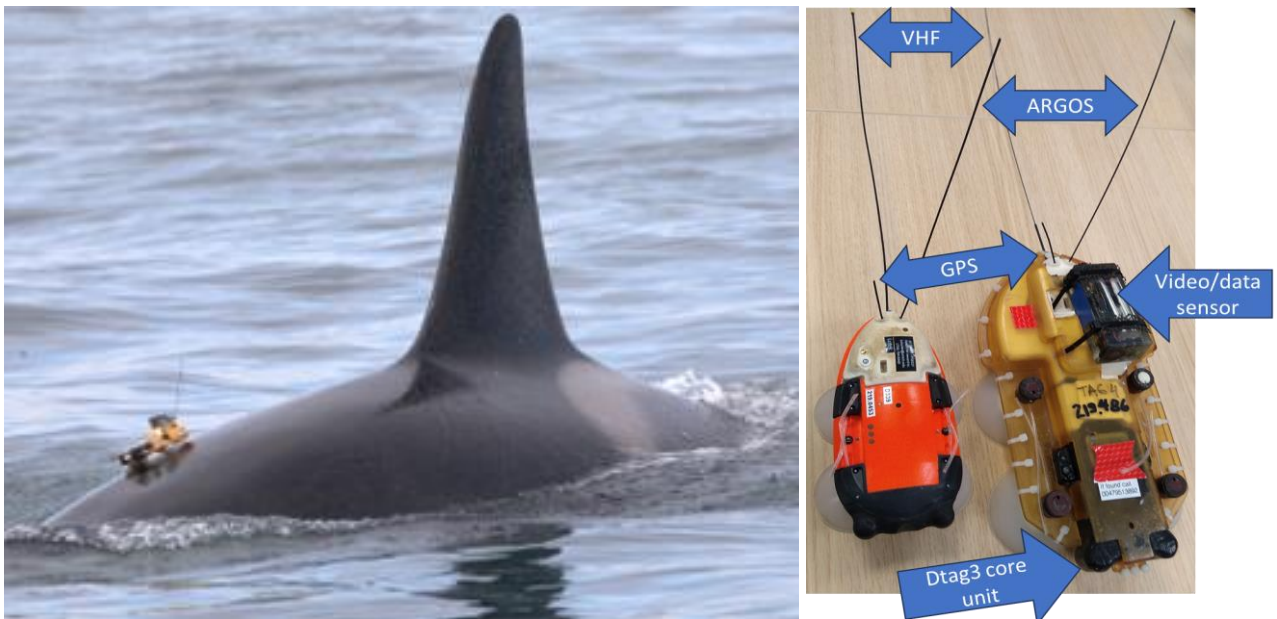
Figure 1: Left panel shows Mixed-DTAG++ deployment oo23_181b. This deployment stayed attached to the whale for 24 hrs, and proved to be the ideal placement for successful goniometer reception of GPS locations. Photo by Anna Selbmann. Right panel shows the two tag types used in trial, integrated-DTAG on the left and Mixed-Dtag++ on the right. Note that the two tag types use the same LOTEK F6G134A FastGPS ARGOS system. The mixed-DTAG++ includes a DTAG3 core unit, and a Little Leonardo DVLW2000M130SW-4R video and data logger.
