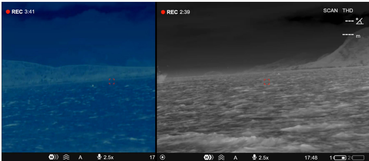
Figure 5. Test of Pulsar Merger LRF XP50 in total darkness. In the left panel a killer whale at 700 m by using ultramarine colour mode, while in the right panel a killer whale at 700 m by using white hot colour mode.
