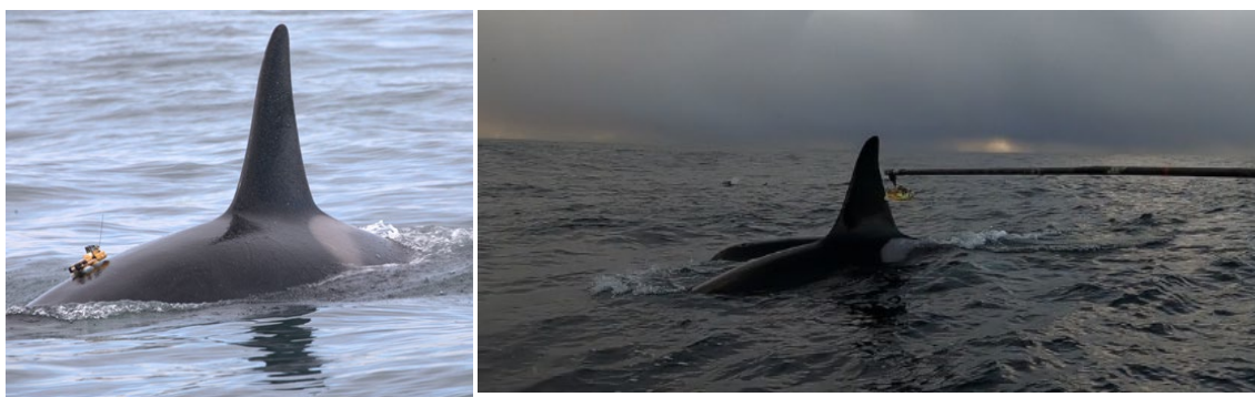
Figure 2.3 Left: Mixed-DTAG ++ deployment Oo23_181b illustrating the optimal placement of the tag for effective performance of the GPS-ARGOS system. Flat placement on the body between the dorsal fin and blowhole. (Photo A. Selbmann). Right: Illustration of the tag-pole setup for attached mixed-DTAG ++ tags by lowering it onto the body between the dorsal fin and the blow hole. (Photo G. Sato).
