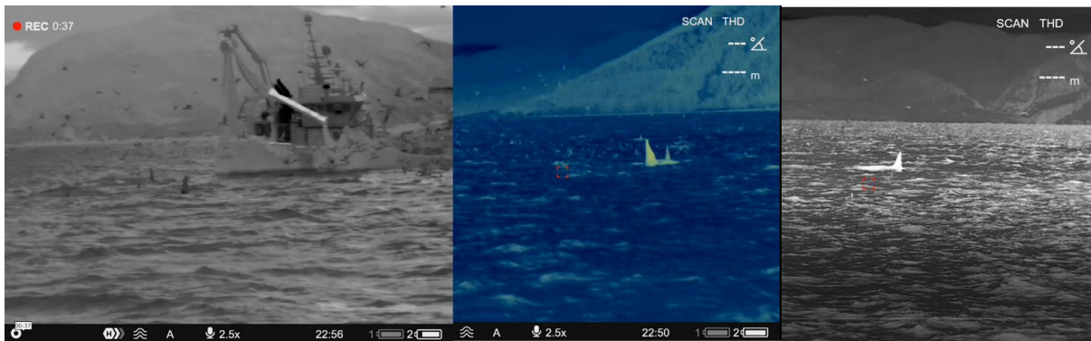
Figure 4. Test of Pulsar Merger LRF XP50 in total darkness. In the left panel killer whales at 150 m by using black hot colour mode, middle panel killer whales at 150m by using ultramarine colour mode, and in the left panel killer whale at 150 m by using white hot colour mode.
