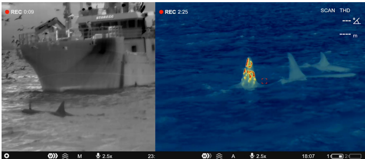
Figure 3. Test of Pulsar Merger LRF XP50 in total darkness. In the left panel a killer whale at 40 m by using black hot colour mode, while in the right panel killer whales at 40 m by using ultramarine colour mode.
