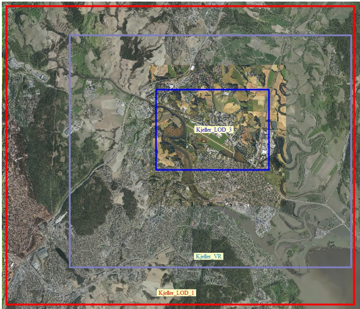
Figure 4.10 The databases are built with two different levels of detail. The red rectangle shows the database area for VR-Forces, and the smaller violet area shows the database area for VR-Vantage with HMD. In both databases, the blue area has a higher level of detail.
