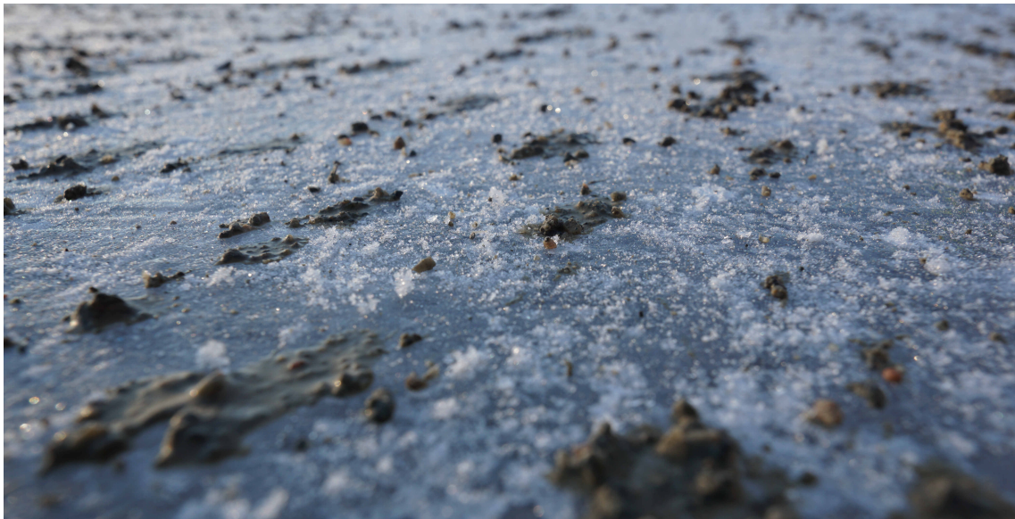
Figure 2.3 Frozen sand test field with Evenes Natural cover sand at Evenes. Photo: FFI.
