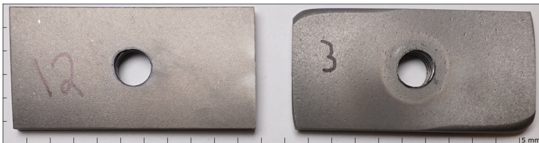
Figure 5.7 F100 blade impeller not used for testing (left) and after completed LCPC Test 1 with Nystad Maskin (right). Photo: FFI.
