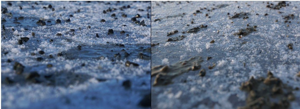
Figure 5.2 Side by side comparison of frozen Crushed Rock (left) and Natural Evenes (right). Beware that the images were taken at slightly different angles and lighting. Photo: FFI.
