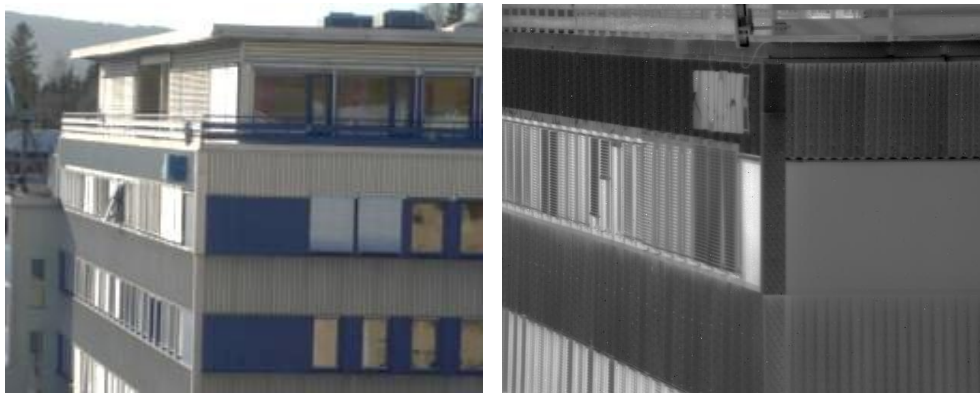
Figure 12. Visual image ( left ) and LWIR image ( right ) of a building vis-à-vis the location of FFI at Kjeller, Norway. LWIR image recorded with the IRCAM camera showing parts of the second and third floor.
