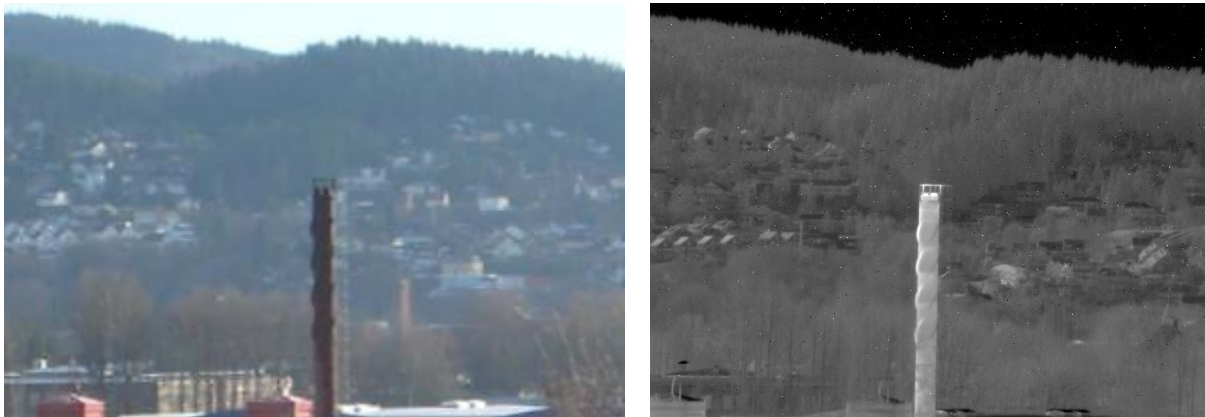
Figure 3. Visual image ( left ) and LWIR image ( right ) of a chimney on a central heating plant at Kjeller, Norway, recorded in March 2014. Field of view is not exactly the same in the two images.
