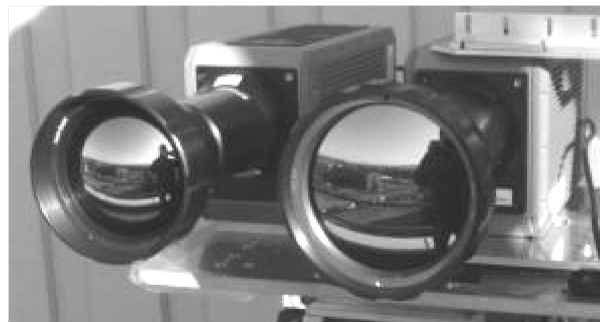
Figure 2. MWE and LW cameras from IRCAM GmbH with 200 mm lenses.
