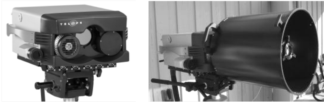
Figure 1. Telops Inc. HyperCam. Left: Instrument with standard optics. Right: HyperCam with 3.5x telescope.
