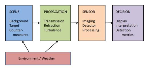
Figure 1: Block scheme of the observation chain
