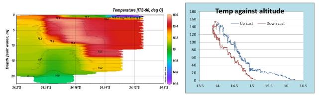
Figure 5: Left panel: sea water temperatures along path from IMT to St. James; Right panel: Vertical profile of air temperature acquired with the helikite.
