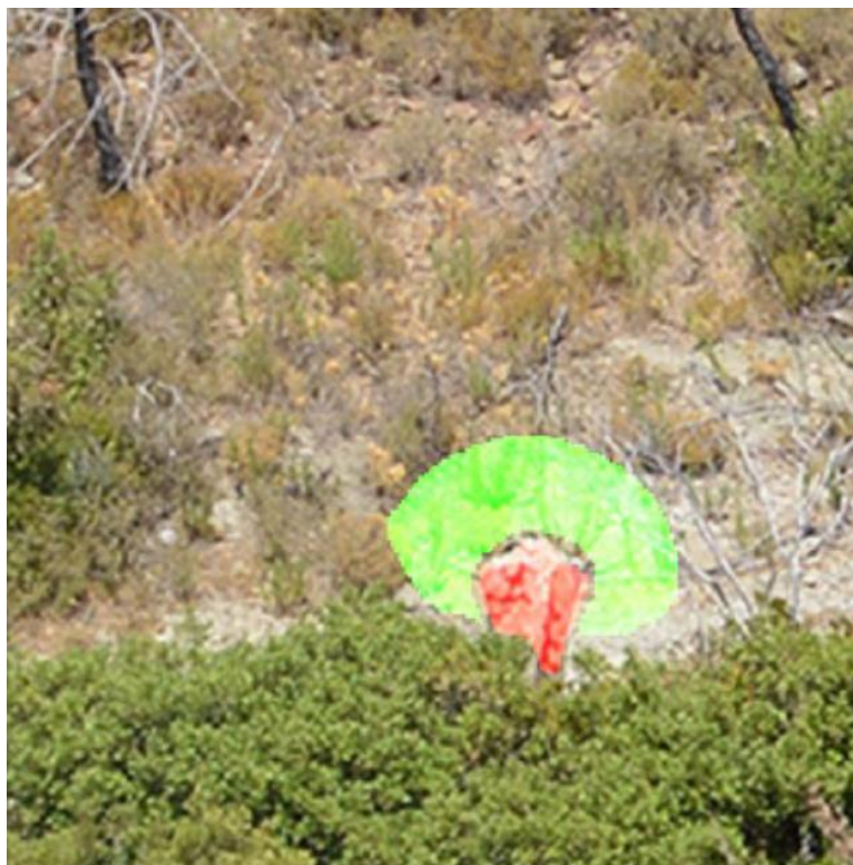
Figure 3. Illustration on how one of the targets was marked (red) in scene 2 for further use by CAMAELEON. The green halo above and to either side of the target shows one of our 5 differently chosen local backgrounds, to which the targets were to be compared, in order to find an estimate on the targets detectability, given in metres.
