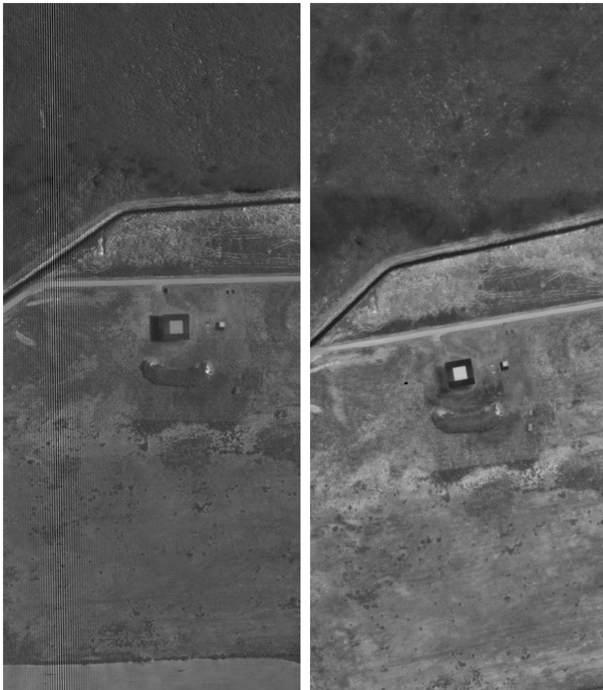
Figure 4. left: MWIR interferometric image from SIELETTERS (note the interference fringes on the left). Right: LWIR panchromatic image for MTF estimation (see section 3.2). This image is acquired during another flight in different conditions.
