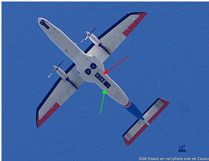
Figure 1. The DO-228 of the DLR with the hatch opened ( 200\text{cm} \times 50\text{cm} ). The 2 circles (red arrow) are the LWIR and MWIR SIELETTERS components, the black rectangle (green arrow) is the Hyspex ODIN instrument.
