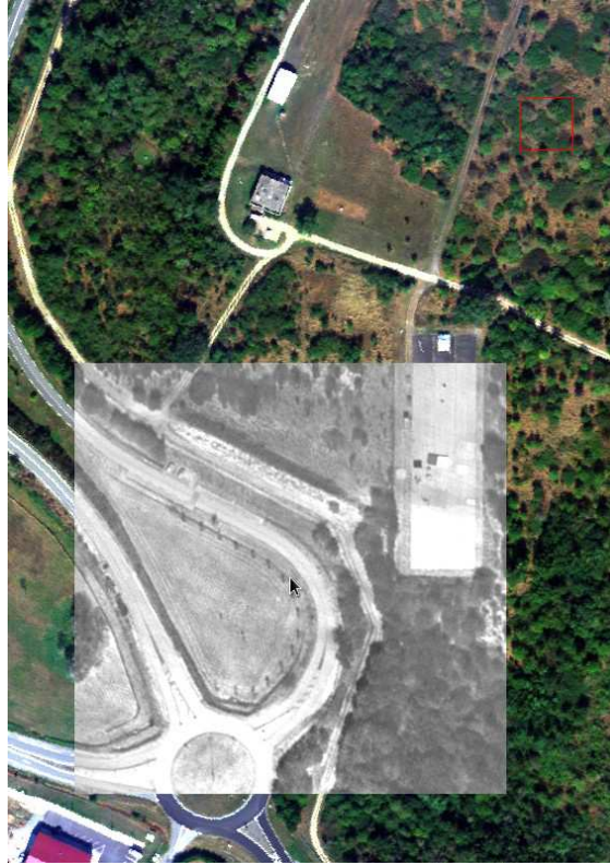
Figure 16 : STAD registration result illustration by superimposition of the 4.7 \mu\text{m} spectral band over a RGB image of ODIN spectral image
