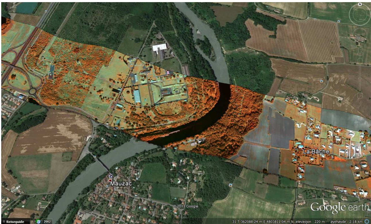
Figure 3. RGB georeferenced image acquired by HySpex ODIN-1024 represented on the GoogleEarth map.
