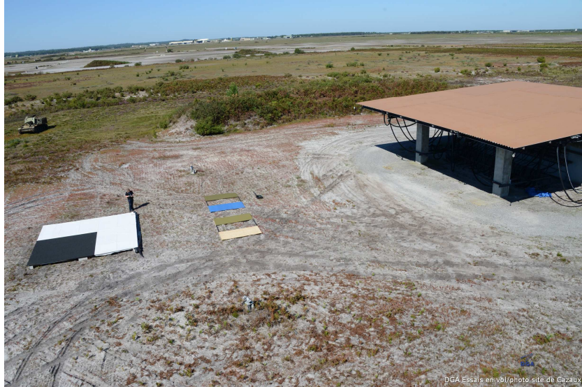
Figure 7. The Cobra target at Cazaux on the right (active infrared target), Black and white target reflective target on the left, different kind of material target in the middle.
