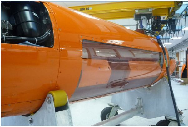
Fig. 2. The HISAS 1030 interferometric SAS mounted on a HUGIN 1000-MR autonomous underwater vehicle.
