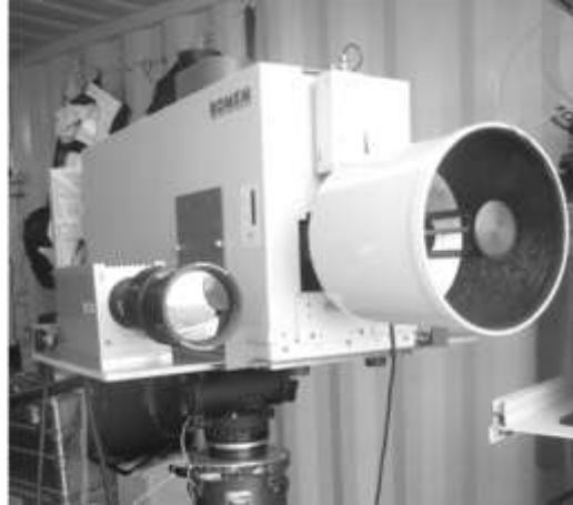
Figure 2. The Cedip MWIR camera used during the trial. The other, larger instrument in the image is a high-resolution radiometric FTIR instrument.
