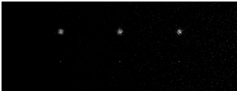
Figure 5. Adherence statistics filtered version of figure 2, with estimated background subtraction. The background noise is significantly suppressed.
