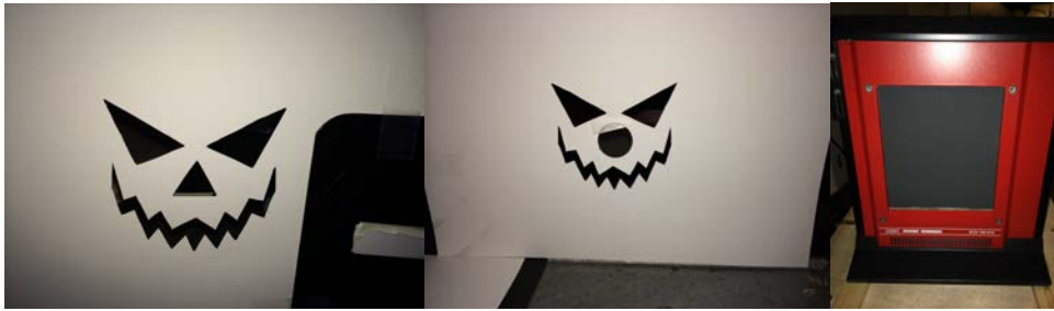
Figure 5. Halloween mask without (left) and with (middle) a Germanium substrate on the nose. The mask was put in front of a black body (right) operated at 300^\circ\text{C} . The mask was cooled down to room temperature using a regular fan.
