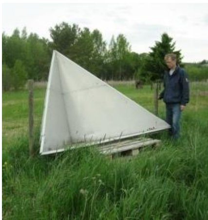
Fig. 2. Radar corner reflector at Kjeller airport. Photo: D. J. Weydahl, FFI.
