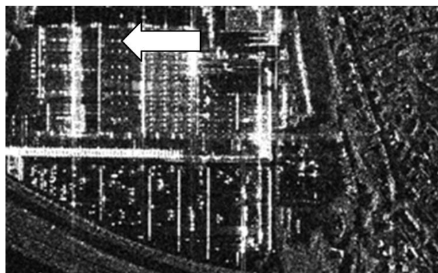
Fig. 4. Norwegian Trade Fair building in Lillestrøm, Norway. A subset of the TSX images acquired over Lillestrøm with 54^\circ (upper image) and 47^\circ (lower image) incidence angles. Note the trapdoor windows on the roof showing up as bright backscatter spots in the SAR images. The spots marked with a white arrow on the western part of the roof are used to estimate the roof height, see also corresponding photo on the very top of Figure 3. Copyright SAR data: TSX 2008, DLR.
