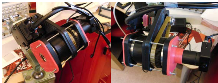
Figure 7. IR TOSCA camera, seen from two angles. The unit consists of, from left to right: Lens holder (red), roller bearing fixture (black), roller bearing (steel), periscopic mirror holder with circular aperture (black, circular barrel), 21-slot air gap reticle (black rounded square shape), motor fixture with motor (black), periscopic mirror holder with toothed wheel incorporated (black, connected to the motor toothed wheel), roller bearing (steel), collimator lens holder with press fit tube for lens/detector assembly (red), detector/lens assembly (black).
