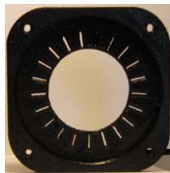
Figure 6. IR TOSCA reticle, printed with the 3D printer. The reticle incorporates the fixture frame with mounting holes leading to an automatic centering of the mask. As seen, not all the 21-slot air gaps are open, so a grinding process was necessary to produce acceptable slits. A simple hand tool was found sufficient.
