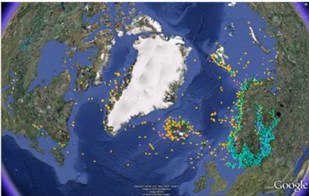
Figure 1.2 The first AIS data from AISSat-1. The yellow and orange symbols show the new AIS data that the satellite gives in addition to the data from the land-based network shown in turquoise symbols.
