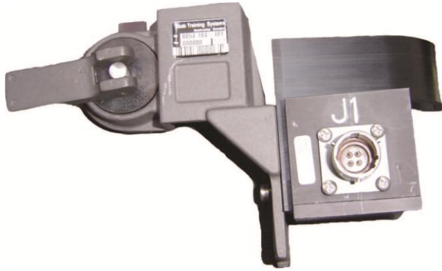
Figur 5.19 Turret Position Sensor [8]
