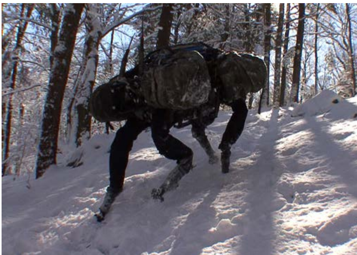
Figure 2.12 BigDog is an example of a UGV under development that can carry equipment and supplies for dismounted soldiers in rough terrain. It is at the foundation of DARPA's recent prototype Legged Squad Support System, LS3 [17] (photo: Boston Dynamics).
