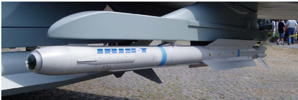
Figure 5.12 IRIS-T short range air-to-air missile with an IR-seeker (photo: Wikimedia Commons).
