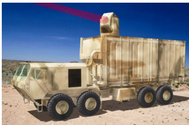
Figure 10.2 Illustration of the High Energy Laser Technology Demonstrator (source: Boeing).
