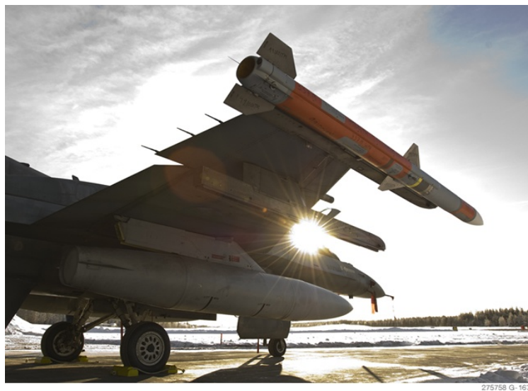
Figure 5.10 F-16 with an AIM-120 AMRAAM on its wing tip station (photo: Raytheon).
