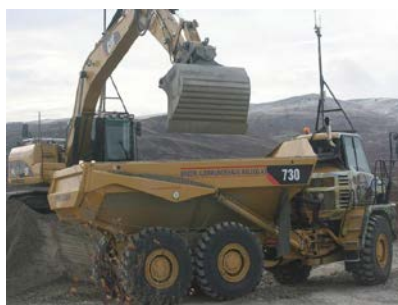
Figure 2.14 Left: Three trucks with one lead driver conducting a test in 80 km/h (photo: NEDO). Right: Remotely controlled shovel and dumper at Hjerkins firing range (photo: Geir Olav Slåen).
