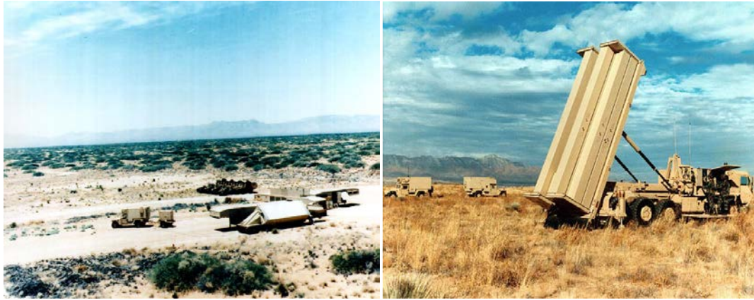
Figure 2.10 THAAD radar installation to the left and a missile launcher to the right (source: fas.org).
