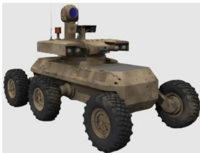
Figure 2.13 The Armed Robotic Vehicle-Assault-Light (ARV-A-L) infantry support UGV of the now terminated FCS programme with sensors and effectors to take out personnel and armoured vehicles (source: Wikimedia Commons).
