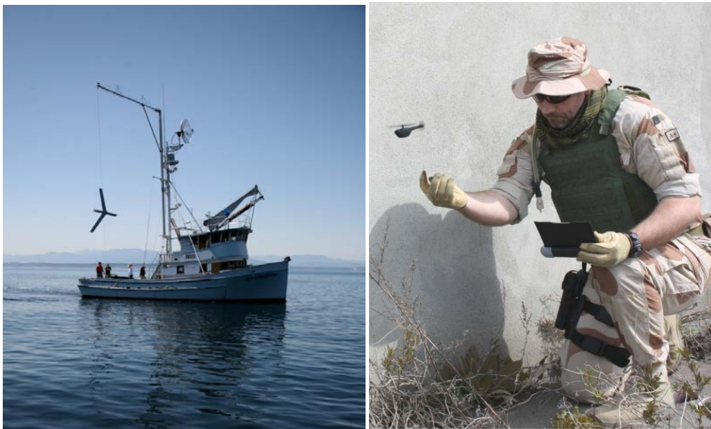
Figure 4.12 Left: Scan eagle from Insitu during landing on a boat (photo: Insitu). In 2010, the US Navy signed contracts within their STUAS programme for deliveries of UASes to some of their smaller vessels. Right: PD-100 from Prox Dynamics is an example of a Nano-UAS (photo: Prox Dynamics).
