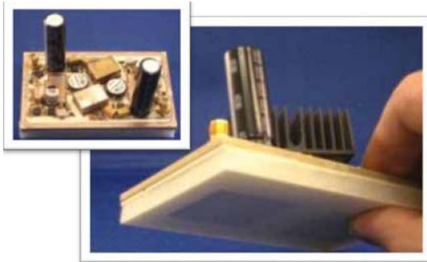
Figure 3.6 Two antenna elements with transceiver module packed in plastic (photos: see [32]).
