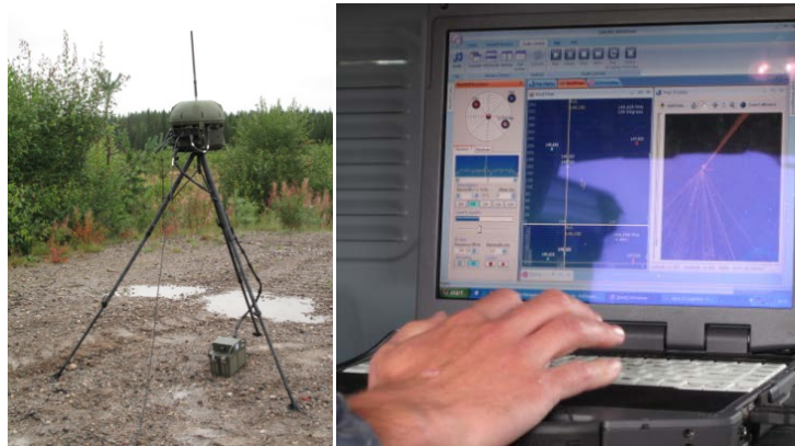
Figure 8.6 Illustration of a modern portable ES sensor (photos: FFI). Left: MEWS sensor, Right: MEWS controller/analysis unit.
