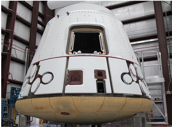
Figure 6.1 The Dragon spacecraft, built by the American company SpaceX, completed the first orbital test in December 2010, orbiting the Earth twice. This spacecraft can take up to 7 astronauts to the ISS, or serve as a cargo transporter (source: see [7]).
