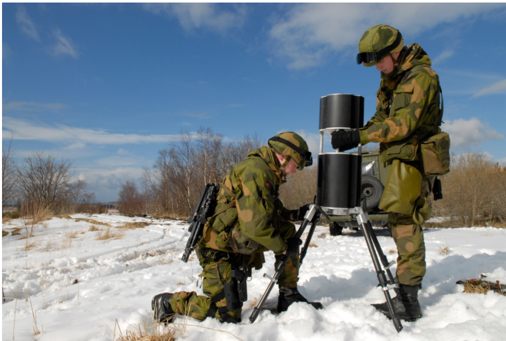
Figure 7.1 CATSS (Chemical, Atomic and Toxic compounds Surveillance System) [88] is an example of how an automatic, network based surveillance system for nuclear radiation, chemical threat agents and toxic industrial chemicals can be built based on existing and available sensors that are put together as required for the operation or situation (photo: FFI).
