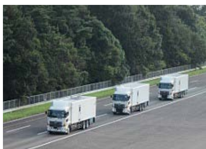
Figure 2.14 Left: Three trucks with one lead driver conducting a test in 80 km/h (photo: NEDO). Right: Remotely controlled shovel and dumper at Hjerkins firing range (photo: Geir Olav Slåen).
