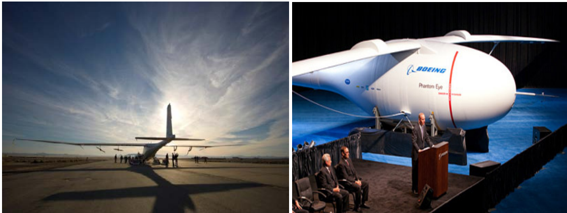
Figure 4.11 Left: Global Observer (photo: AeronVironment Inc.). Right: Phantom Eye (photo: Boeing) are examples of new UASes that can carry considerable payload at high altitudes but are nevertheless able to give an endurance up to a week.
