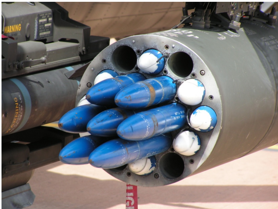
Figure 4.20 Hydra 70 rockets in an M261 launch pod on a Dutch AH-64 Apache on display at the RIAT2007 (photo: Wikimedia Commons).
