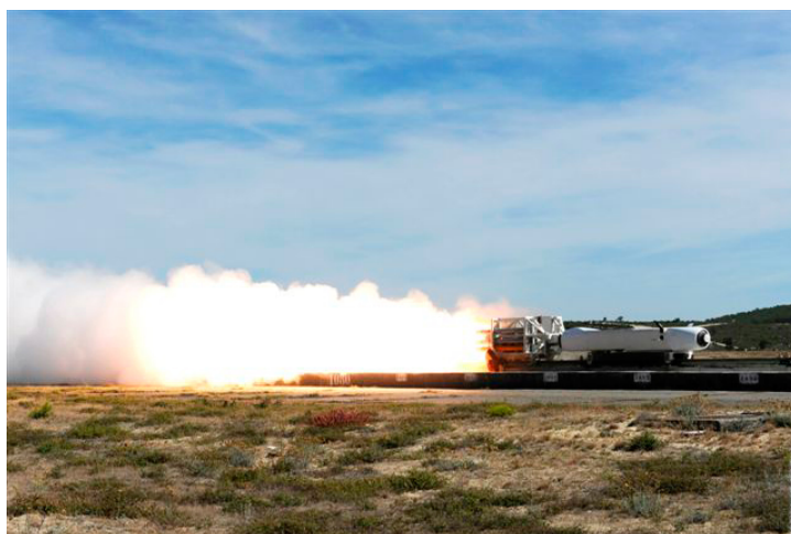
Figure 5.5 Sleigh test of MBDA's new HARDBUT warhead (photo: MBDA).
