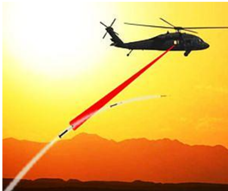
Figure 8.4 Illustration of a DIRCM system in use (source: Raytheon).
