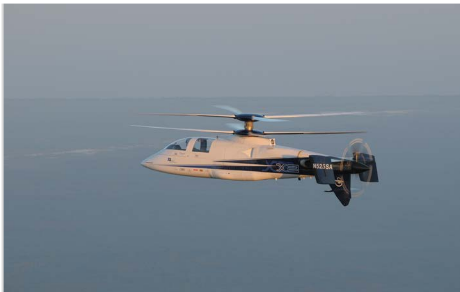
Figure 4.9 Sikorsky X2 is an experimental helicopter with coaxial rotors and auxiliary propulsion (photo: Sikorsky).
