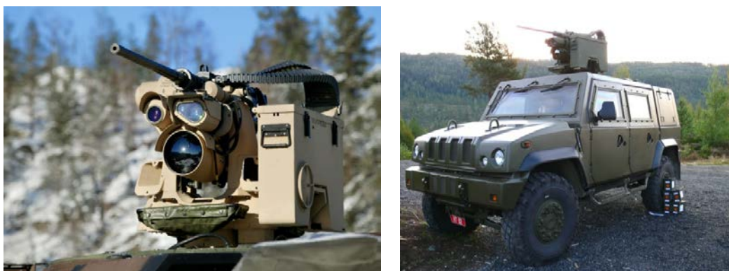
Figure 2.4 Left: Kongsberg's Remote Weapon System, Protector. Right: Protector mounted on an Iveco vehicle (photos: Kongsberg).
