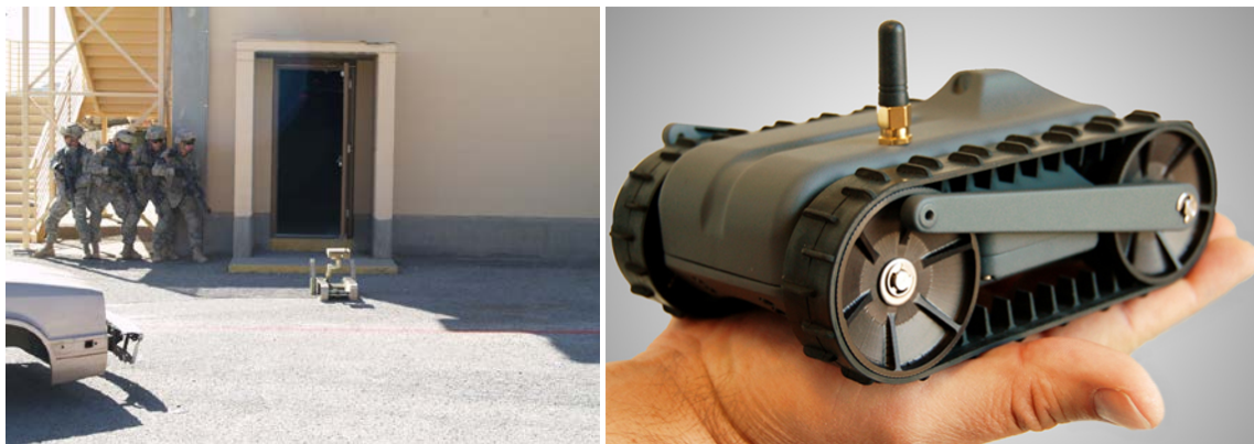
Figure 2.11 Left: SUGV (Packbot) assisting soldiers in operations. Right: LANdroids (photos: iRobot Corporation).
