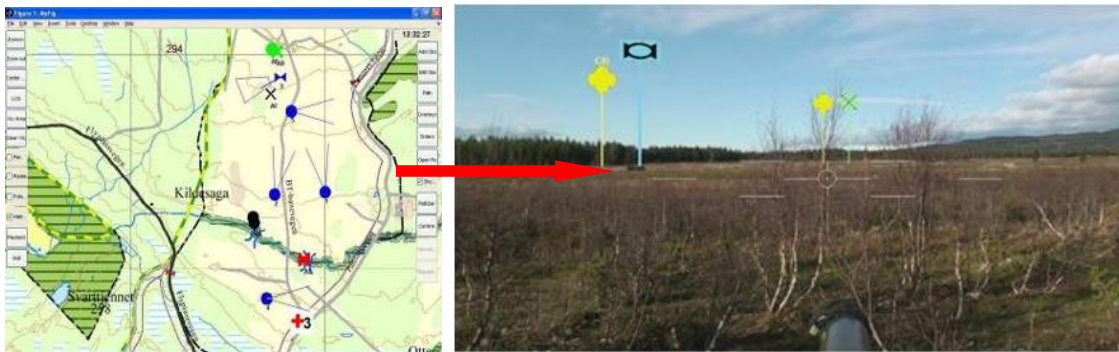
Figure 2.7 Augmented Reality (AR) – Information in BMS is displayed in the image from the day sight of CV90 Infantry Fighting Vehicle (source: FFI).
