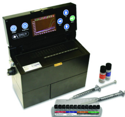
Figure 7.7 RAZOR is a handheld PCR instrument developed by Idaho Technologies (photo: FFI).
