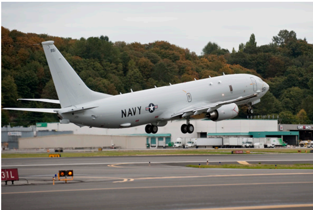
Figure 4.7 P-8 Poseidon is based on the Boeing 737 airframe and will replace the P-3 Orion (photo: Boeing).
