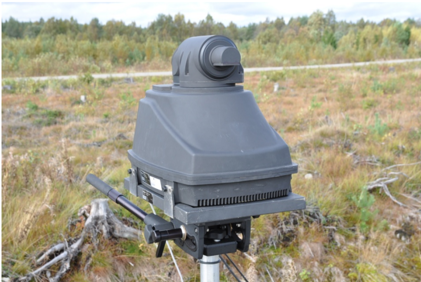
Figure 7.2 Passive Stand-off IR detector Bruker RAPID, range 5 km (photo: FFI).
